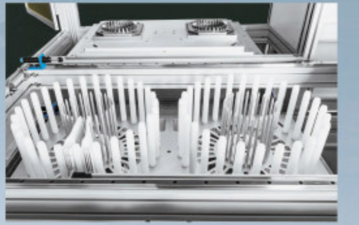
堆叠工装治具 Jig for stacking products
