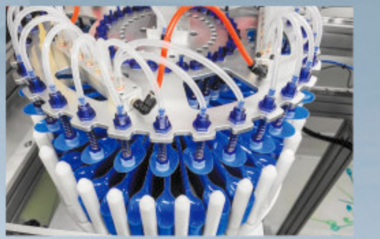
堆叠工装治具 Jig for stacking products
