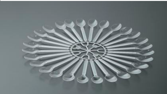
Mould Name: spoon mould Plastic Material: PS Cavities No.: 56 Cavities Part Weight: 7.1g Runner Type: 3 points hot runner Mould Steel: H13
