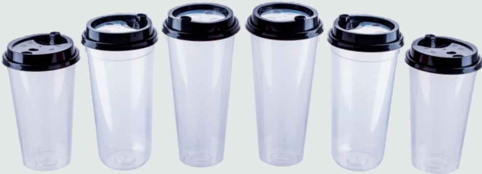
Mould Name: Milk Tea Cup Mould Plastic Material: PP Cavities No.: 8 Cavities Volume: 700ml Cup weight: 22 g Runner Type: Pneumatic valve gate hot runner Mould Steel: 2344
