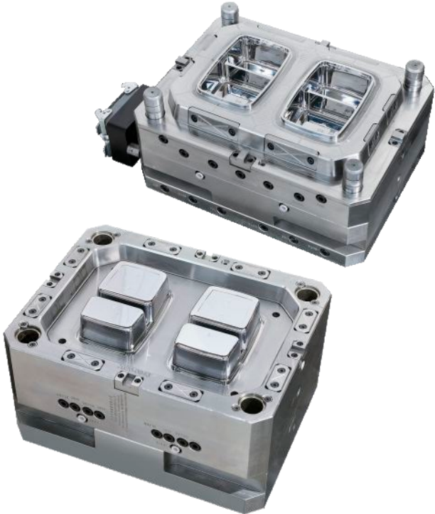
Mould Name: Thin wall container mould Plastic Material: PP Cavities No.: 2 Cavities Part Weight: Container 35 g Lid 15 g Runner Type: full hot runner Mould Steel: 2344
