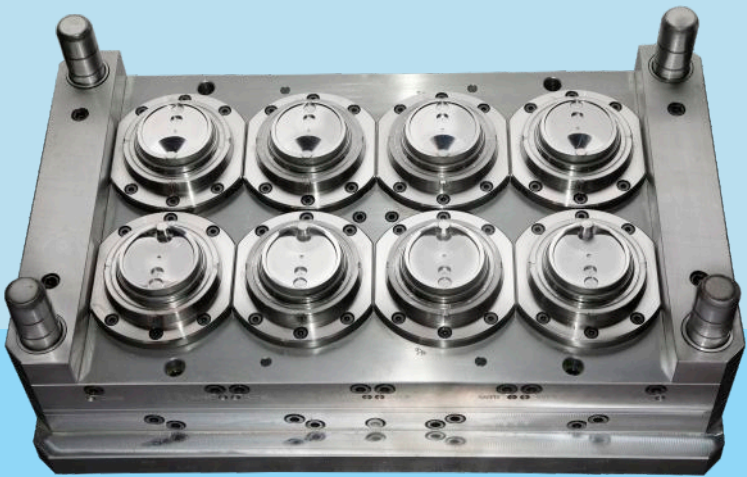
Mould Name: Coffee Lid Cup Mould Plastic Material: PP Cavities No.: 8 Cavities Lid weight: 5.4 g Runner Type: Pneumatic valve gate hot runner Mould Steel: S136
