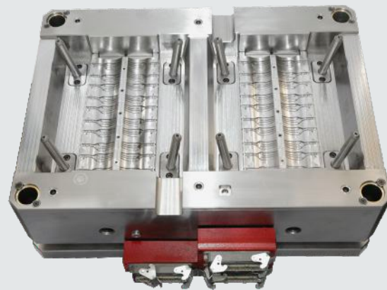
Mould Name: Fold fork mould Plastic Material: PP Cavities No.: 40 Cavities Part Weight: 2.3g Mould Steel: S136
